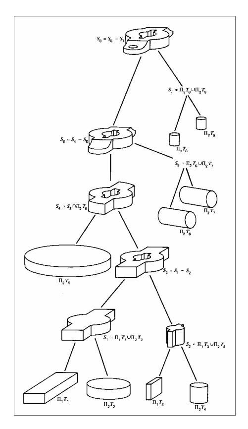
Figure 3. A boolean model of a mechanical part
